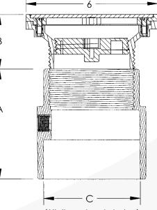
(All dimensions in inches) • Barrel diameter is 3-1/2 in. IPS thread.
